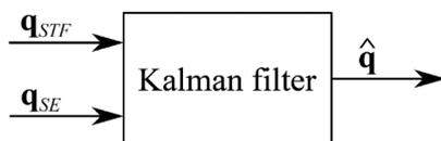
Fig. 5. Linear Kalman filter estimating attitude quaternion
