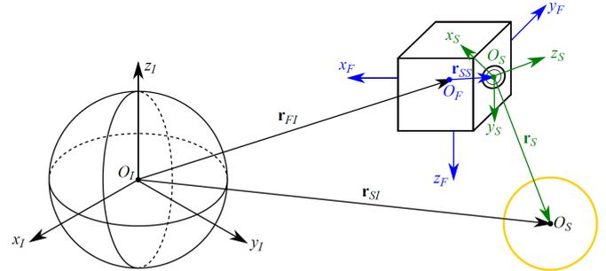
Fig. 2. Sun sensor direction vectors
