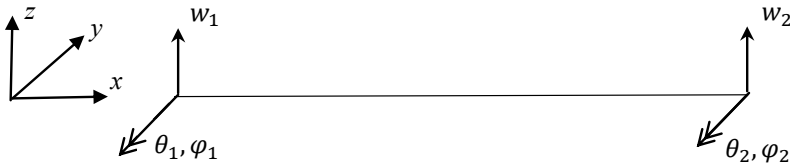
Fig. 5. Finite element model of the Timoshenko beam element
