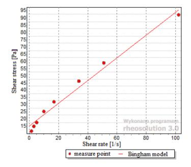
Fig. 2. Yield curve for saline slurry described with Bingham model
