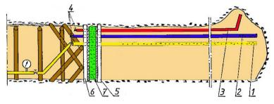
Fig. 1. Schematic of closing end part of working with the pipeline injection method 1 – pumping pipeline, 2 – vent-pumping pipeline, 3 – vent pipeline, 4 – gates, 5 – inner dam, 6 – outer dam, 7 – injection plug
