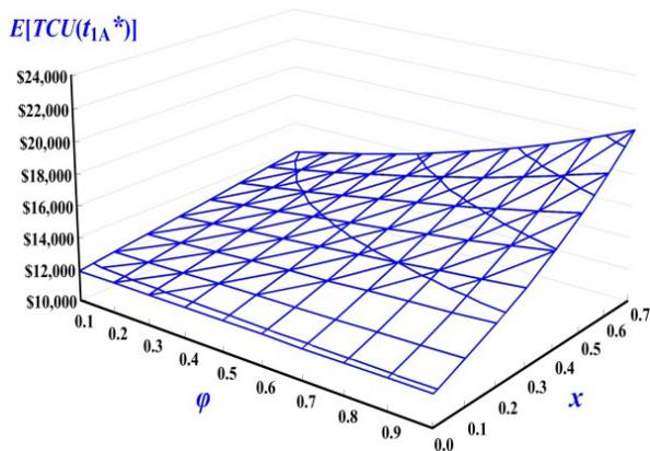
Fig. 15. Joint impact of variations in scrap rate  $\varphi$  and random defective rate  $x$  on  $E[TCU(t_{1A}^*)]$
