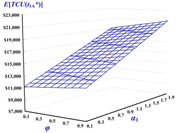
Fig. 17. Joint influence of changes in scrap rate  $\varphi$  and overtime output increase rate  $\alpha_1$  on  $E[TCU(t_{1A}^*)]$
