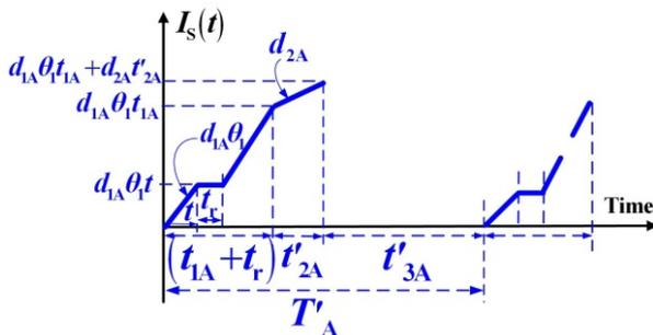
Fig. 4. Level of on-hand scrap items in the proposed EMQ-based system with breakdown occurrence, overtime, and quality-ensured issues
