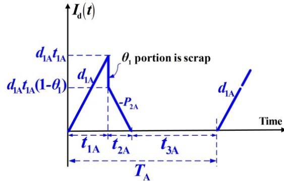
Fig. 7. Level of on-hand defective items in the proposed system without breakdown
