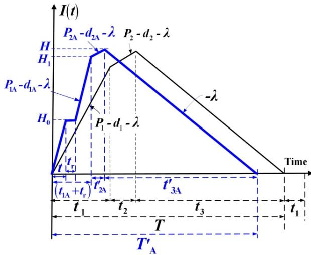
Fig. 1. Level of on-hand perfect stocks in a cycle for the proposed EMQ-based system with breakdown occurrence, overtime, and quality-ensured issues (in blue) as compared to that of a classic EMQ model with quality-ensured issues (in black)
