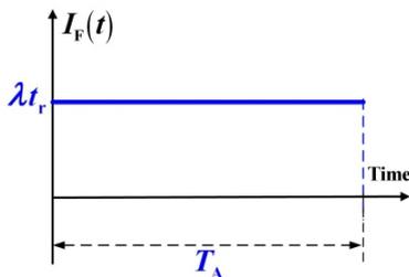
Fig. 6. Level of on-hand safety stocks in the proposed EMQ-based system without breakdown occurrence
