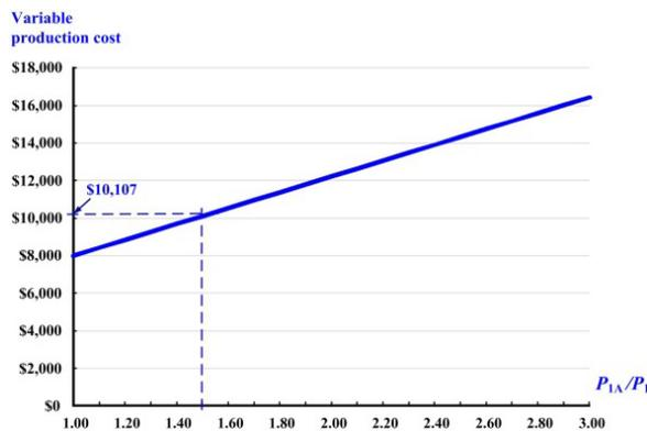
Fig. 11. The effect of differences in overtime relevant ratios  $P_{1A}/P_1$  on variable production cost
