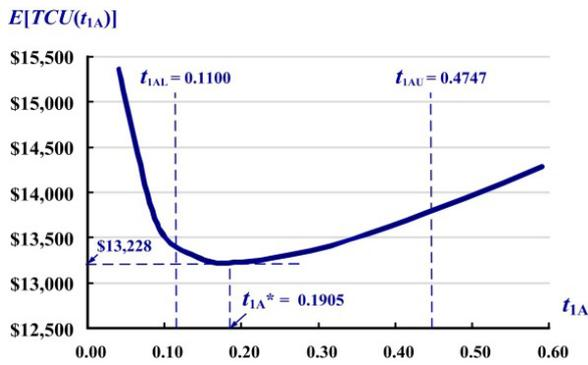
Fig. 9. The effect of variations in uptime  $t_{1A}$  on  $E[TCU(t_{1A})]$
