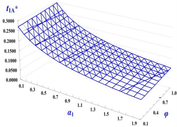
Fig. 16. Combined effect of differences in overtime output increase rate  $\alpha_1$  and scrap rate  $\varphi$  on  $t_{1A}^*$
