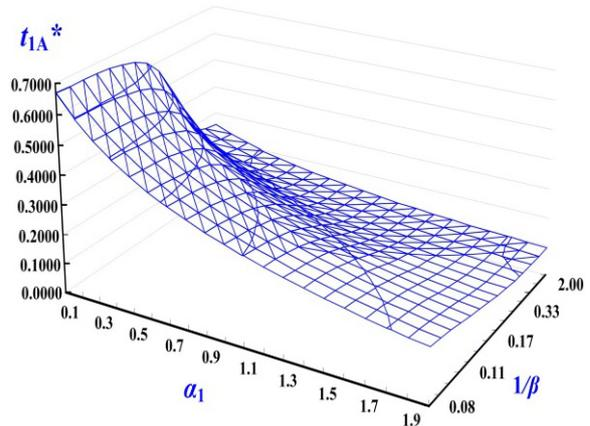
Fig. 18. Combined impact of variations in overtime factor  $\alpha_1$  and time-to-machine-failure  $1/\beta$  on  $t_{1A}^*$
