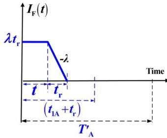
Fig. 2. Level of on-hand safety stocks in the proposed EMQ-based system with breakdown occurrence, overtime, and quality-ensured issues
