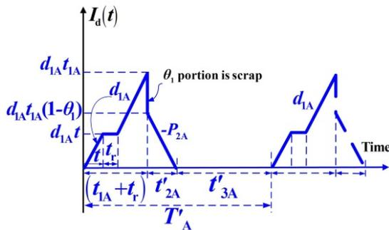
Fig. 3. Level of on-hand defective items in the proposed EMQ-based system with breakdown occurrence, overtime, and quality-ensured issues
