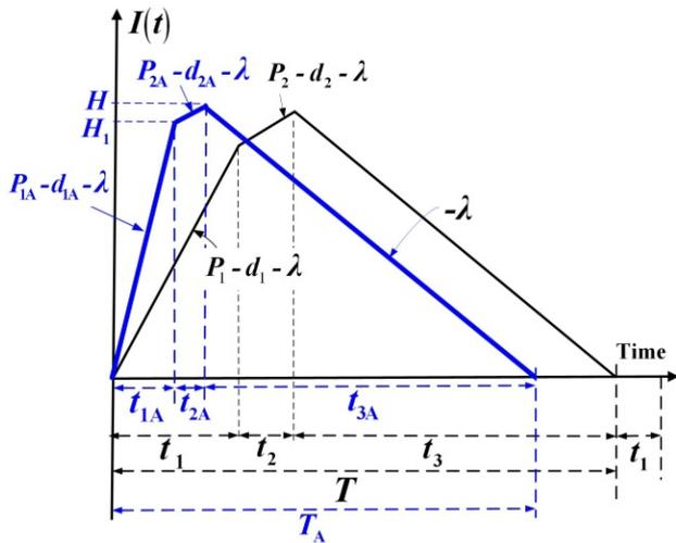
Fig. 5. The level of on-hand perfect stocks in an EMQ-based model with overtime and quality-ensured issues, but without breakdown occurrence (in blue) as compared to that of an EMQ-based model with quality-ensured issues (in black)
