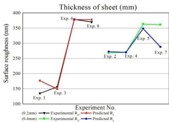
Fig. 9. Comparative results of sheet thickness (T)
