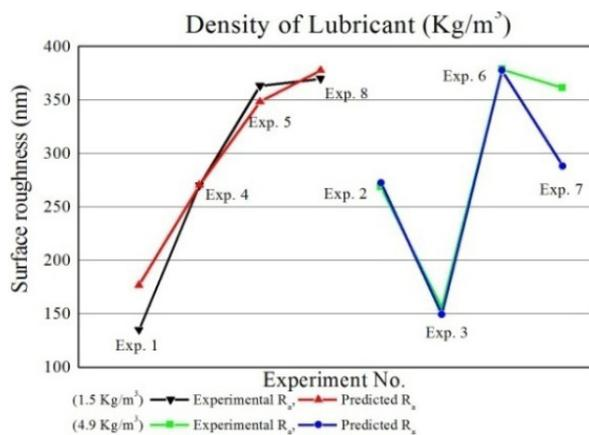
Fig. 10. Comparative results of the lubricant (L)
