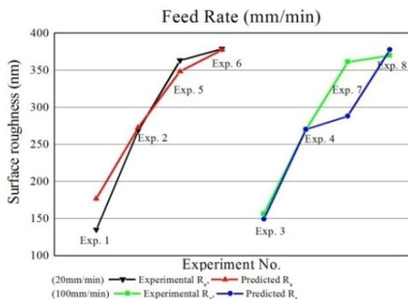
Fig. 6. Comparative results of feed rate (f)
