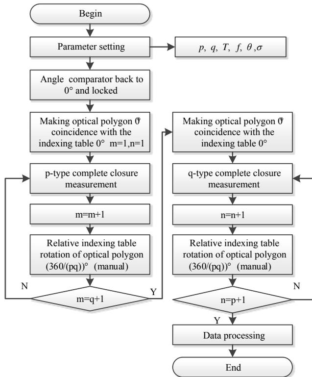
Fig. 2. Experiment Process.
