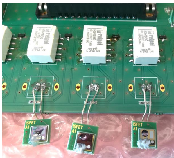
Fig 7. ISFET transistors with applied biological substance
