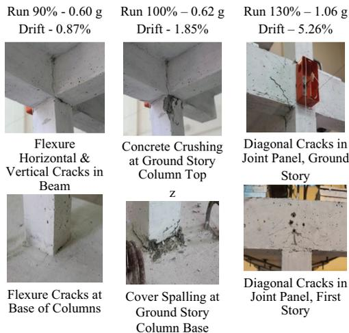
Fig. 4. Code design Model-1 damage response
