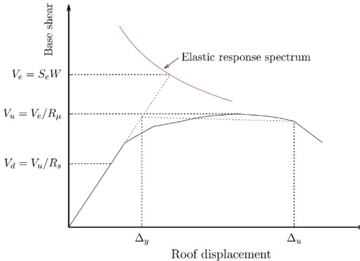
Fig. 12. Response modification factor parameters from capacity curve [31]
