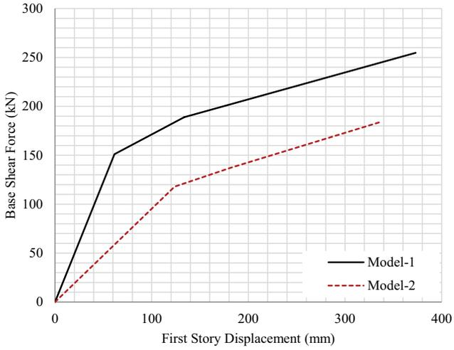
Fig. 8. Prototype frame force-deformation capacity curves
