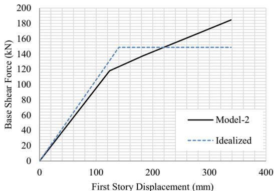
Fig. 10. Model-2 Idealization of force-deformation capacity curve
