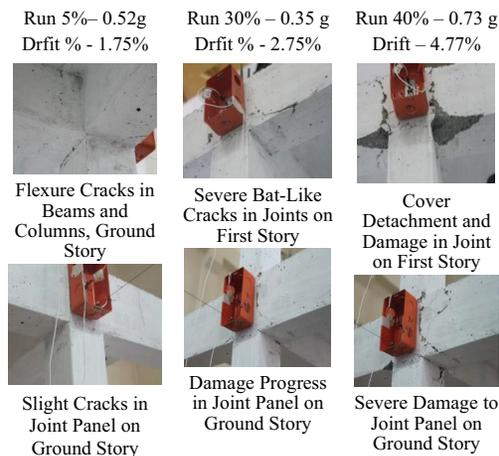
Fig. 5. Deficient weak beam-column joint Model-2 damage response
