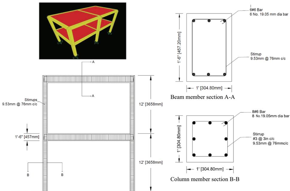
Fig. 1. Layout of two-story frame model, geometry and members design details
