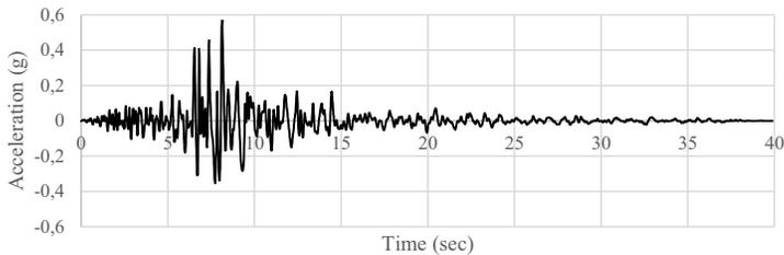
Fig. 3. Input shaking record of 1994 Northridge Earthquake
