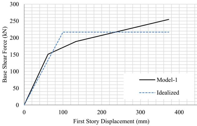
Fig. 9. Model-1 Idealization of force-deformation capacity curve
