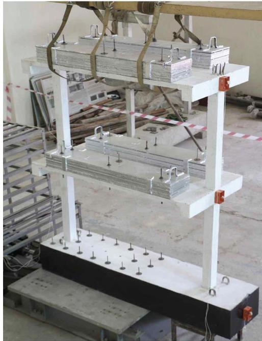
Fig. 2. Test models setup on shake table
