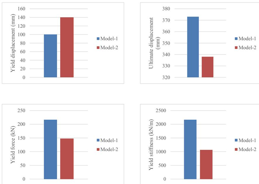
Fig. 11. Response parameter from idealized force-displacement relationships
