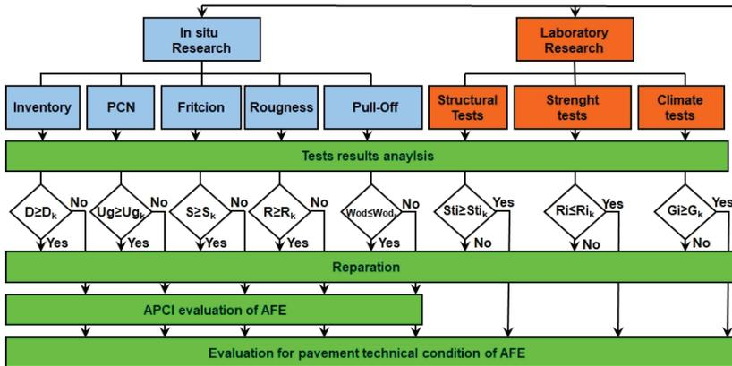
Fig. 1 Assessment of the airport pavement technical condition with the APCI method procedure (PCN – load bearing capacity as a Pavement Classification Number, AFE – Airfield Functional Element)
