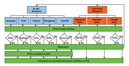
Fig. 1 Assessment of the airport pavement technical condition with the APCI method procedure (PCN – load bearing capacity as a Pavement Classification Number, AFE – Airfield Functional Element)
