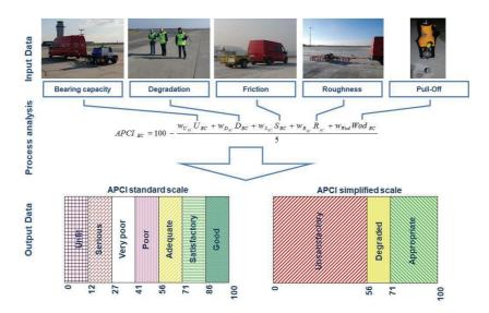
Fig. 2 Assessment of the airport functional element's surface condition with the APCI method
