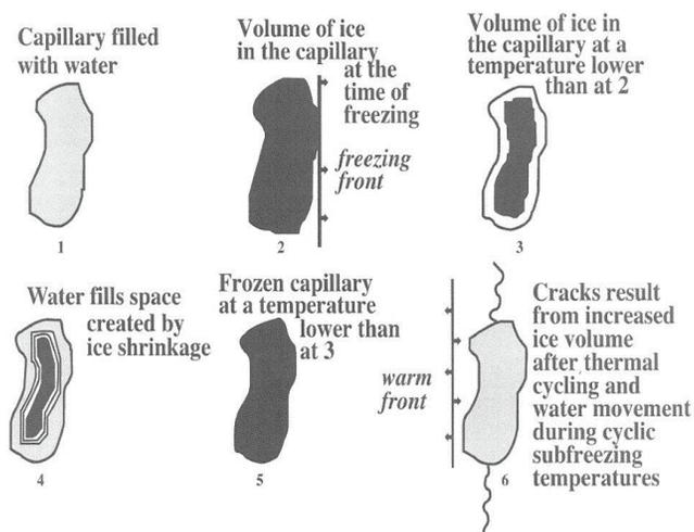
Fig.10. Response of water and ice in a capillary pore in cement paste at the freezing temperature decreases (Erlin & Mather, 2005, also in [20])
