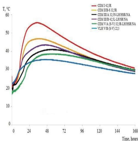
Fig. 3. Relative increase in concrete temperature when using different cements, starting from cements with high heat release kinetics to cements with the lowest calorific value
