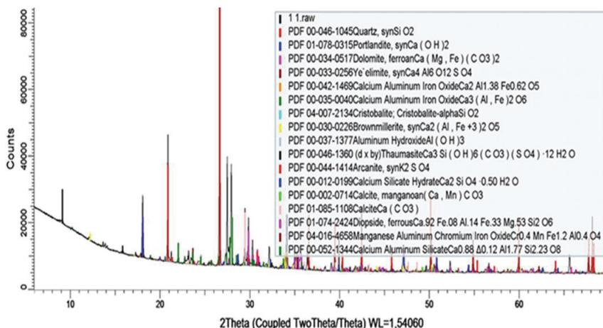
Fig.9. XRD analysis for sample No.1 taken from the near surface layer
