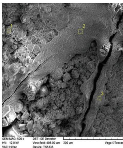
Fig. 4. Image of micro cracks in bridge concrete made with the cement 52,5 R
