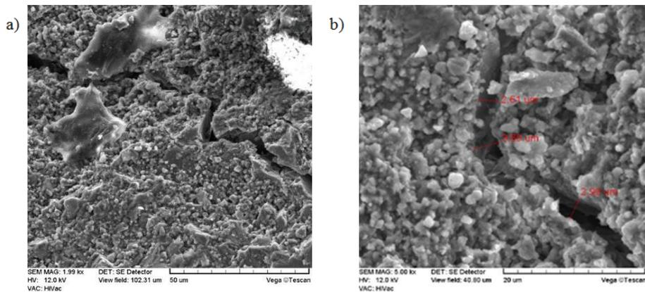
**Fig. 6** Micro cracks of a frozen sample. Drawing (a): magnification 2000 x, observation field 100x100  $\mu\text{m}$ . Drawing (b): magnification 5000 x, observation field 40x40  $\mu\text{m}$ ; width of the cracks between 2.61 and 3.69  $\mu\text{m}$
