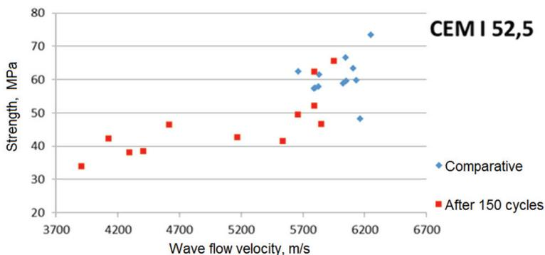
Fig. 2 Relation of the ultrasonic wave flow velocity - concrete compressive strength of Ø100 mm well samples taken from road viaducts ( details in [16])
