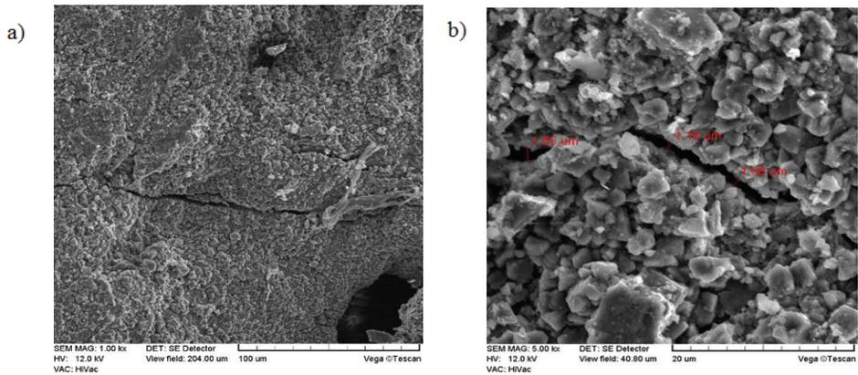
**Fig. 5** Micro cracks of an unfrozen sample. Drawing (a): magnification 1000 x, observation field 200x200  $\mu\text{m}$ . Drawing (b): magnification 5000 x, observation field 40x40  $\mu\text{m}$ ; width of the cracks from 1.08 to 1.65  $\mu\text{m}$
