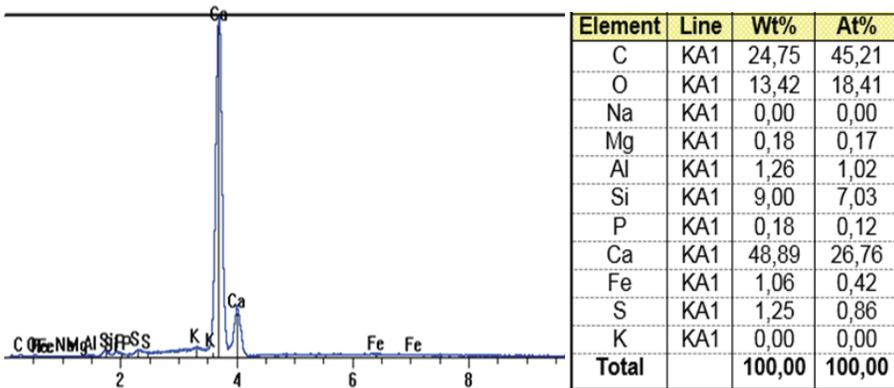
Fig. 8 Chemical composition of cracks from Fig. 7 – b. Note the very large amount of calcium and carbonates
