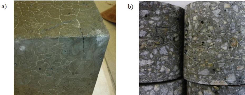
Fig. 1 Grid micro cracks filled with white salt sediment on both samples 15x15x15 cm taken during the concreting of the viaducts (a), as well as cylindrical samples Ø100 mm cut from the flyover structure (b)
