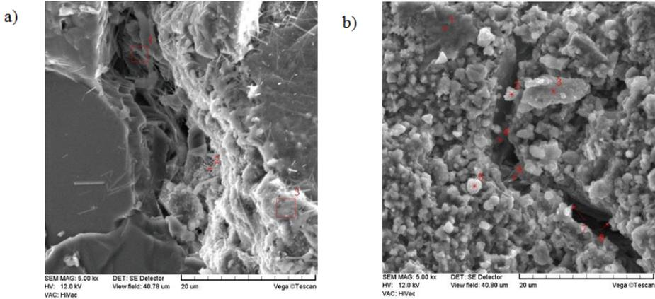
Fig. 7. Micro cracks (a) and their filling(b)
