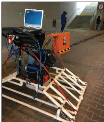
Figure 4. Measurements of the bottom slab of the tunnel with 1.0 GHz air-coupled antenna and 400 MHz ground-coupled antenna. To conduct investigations with two antennas at the same time, a special trolley was prepared.
