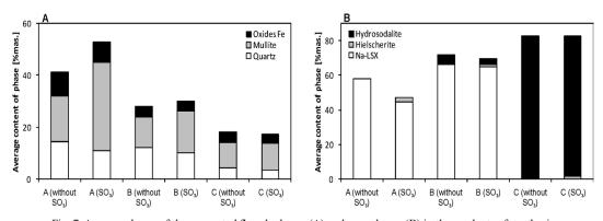
Fig. 7. Average shares of the unreacted fly ash phases (A) and new phases (B) in the products of synthesis by population of sample (samples A, B and C)
