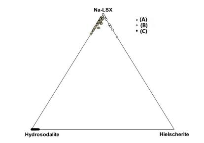
Fig. 5. Projection points of the studied micro-areas in the new phase system of the Na-LSX type zeolite – hydrosodalite – hielscherite according to samples A, B and C
