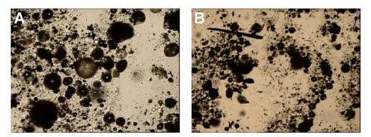
Fig. 1. Microscopic image of the tested fly ash, light passing through one Nicol prism,  $200 \times$  magnification, (A) in the center a spherical enamel aggregate with mullite, (B) elongated grains of opaque organic matter
