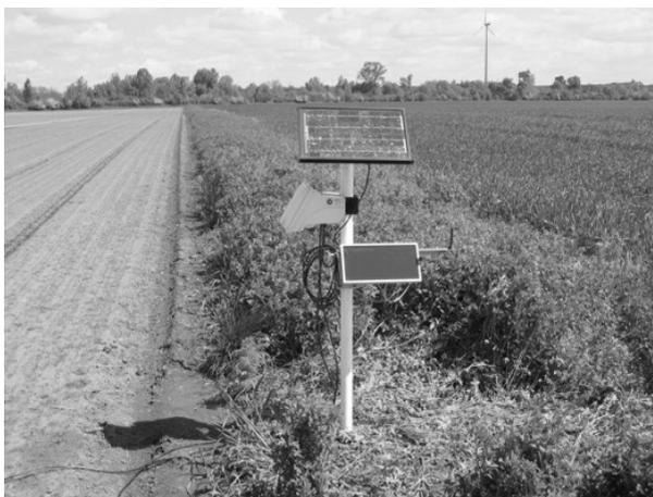
Fig. 2. Soil moisture measurement: logger station from Sentek's EnviroSCAN and GSM modem
