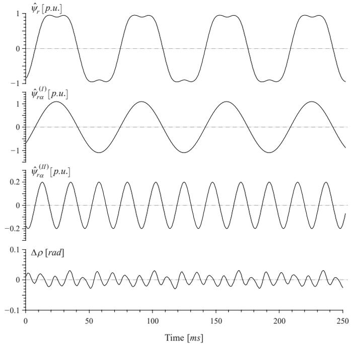
Fig. 5. Rotor flux vector components – resulting rotor flux, rotor flux vector component in 1<sup>st</sup> and 2<sup>nd</sup> plane, and synchronisation error
