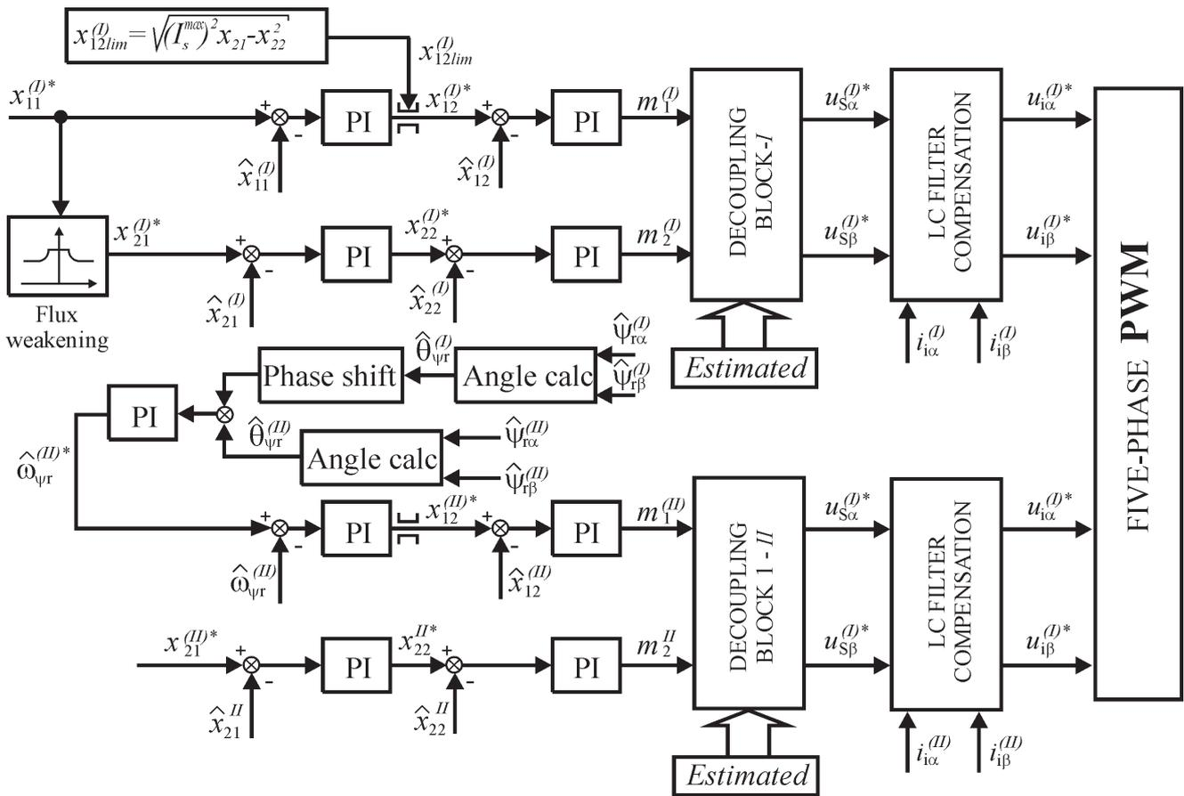
Fig. 3. Multiscale control structure with 3<sup>rd</sup> harmonic injection and rotor flux synchronisation
