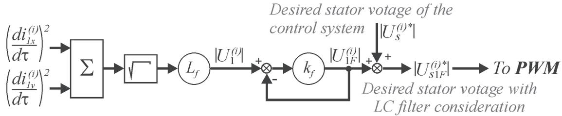
Fig. 4. LC filter inductance voltage drop compensation used in control system
