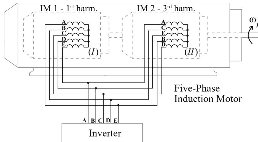
Fig. 2. Schematic representation of the concept of five-phase induction motor control with 3<sup>rd</sup> harmonic injection
