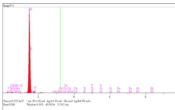
Fig. 8. Chemical composition in the first point on the surface of the sample
