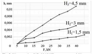
Fig. 2. Linear strain of "Stahl 1018" structure vs. axial impact at temperature 20°C
