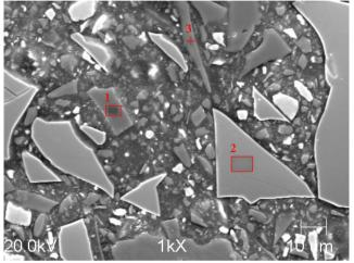
Fig. 3. Microstructure of sample no. 1 performed of MM "Stahl1080" material, obtained with SEM
