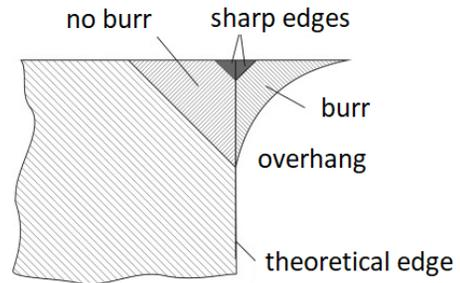
Fig. 2. Scheme of burr according ISO 13715 [22]
