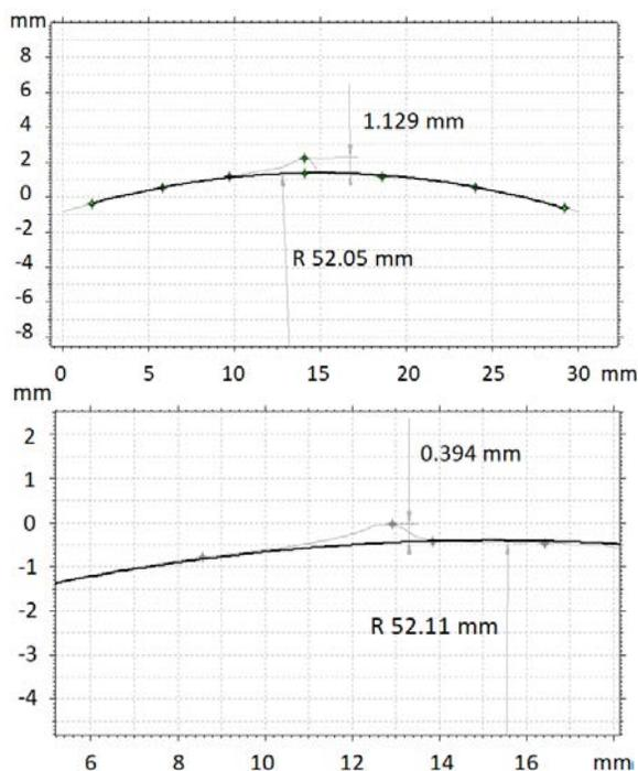
Fig. 6. Surface profile: a) before and b) after flash removal through vibratory machining
