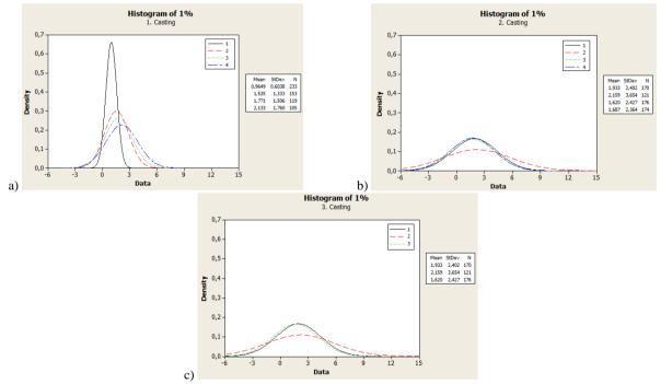
Fig. 6. Density distribution function of pores measured on the cross-section of reduced pressure test samples 1 wt% Ti added and recycled A356: a) 1<sup>st</sup> recycling, b) 2<sup>nd</sup> recycling, c) 3<sup>rd</sup> recycling
