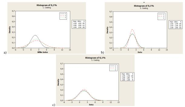
Fig. 5. Density distribution function of pores measured on the cross-section of reduced pressure test samples 0.1 wt% Ti added and recycled A356: a) 1<sup>st</sup> recycling, b) 2<sup>nd</sup> recycling, c) 3<sup>rd</sup> recycling
