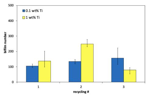
Fig. 3. Number of bifilm change of 3 times recycled A356 with 0.1 and 1 wt% Ti
