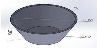
Fig. 1. Dimension of RPT steel cup
