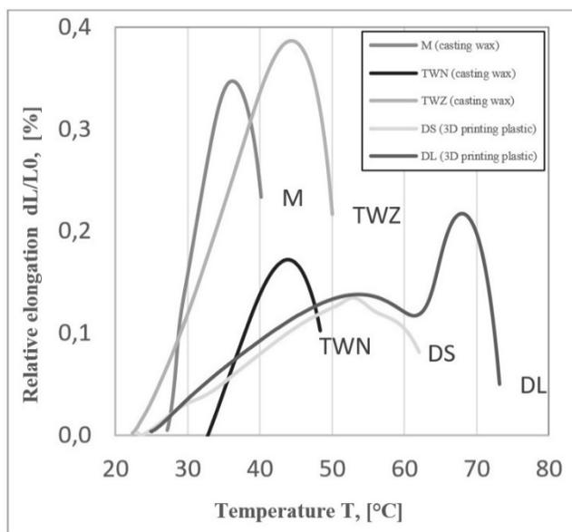
Fig. 1. Changes in relative elongation of foundry pattern materials as a function of temperature
