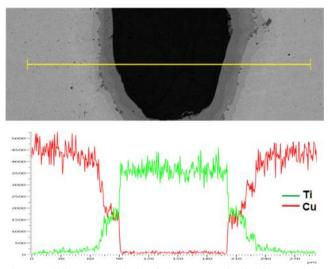
Fig.5. EDS line scan analysis of phases around a titanium particle
