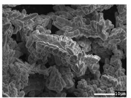
Fig.1. Electrolityc copper powder (SEM)
