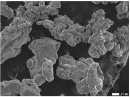
Fig.2. Titanium powder (SEM)
