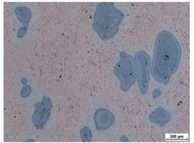
Fig.3. Microstructure of sintered compact obtained for Cu+ 5 % of Ti
