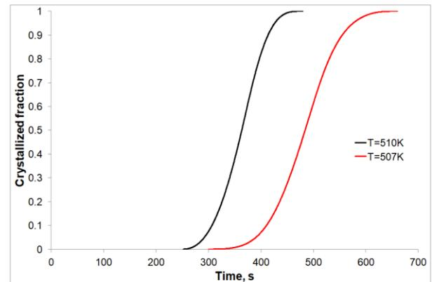
Fig. 6. The crystallized volumetric fraction as a time function for various isothermal annealing temperatures of Mg72Zn24Ca4 alloy
