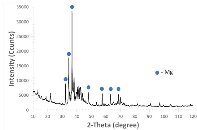
Fig. 2. Results of X-ray diffraction for Mg<sub>72</sub>Zn<sub>24</sub>Ca<sub>4</sub> ribbon after isothermal annealing at 507 K
