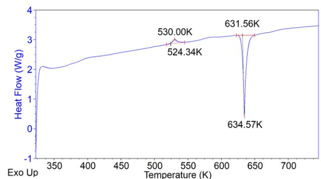
Fig. 3. The course of the ribbon heating to 450 °C with a rate of 5 K / min
