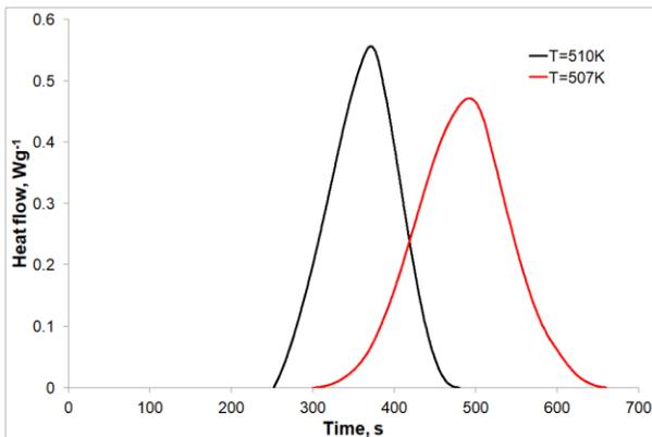
Fig. 4. Isothermal DSC curves traces at different annealing temperature
