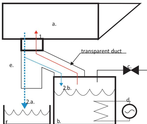
Figure 5: Scheme of the steam generators: a – condensation hood; b – water tank (or combi-steamer); c – water supply valve; d – electric immersion heater; e – SDF; f – condensate container; 1 – steam; 2 – condensate.
