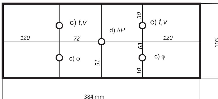
Figure 3: Outlet channel cross-section with location of measurement points:  $t$  – temperature;  $v$  – velocity;  $\varphi$  – relative humidity;  $\Delta P$  – velocity (Pitot tube).
