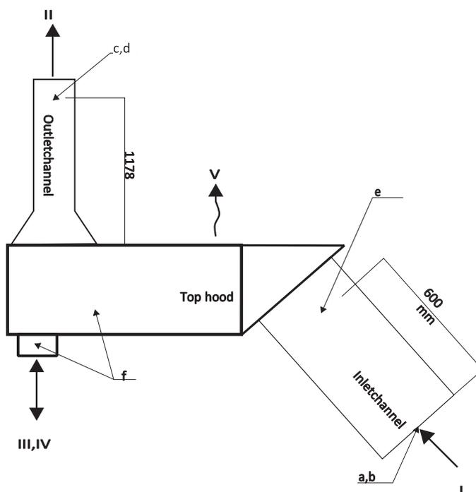
Figure 2: The hood's inlets, outlets and locations of measuring points.
