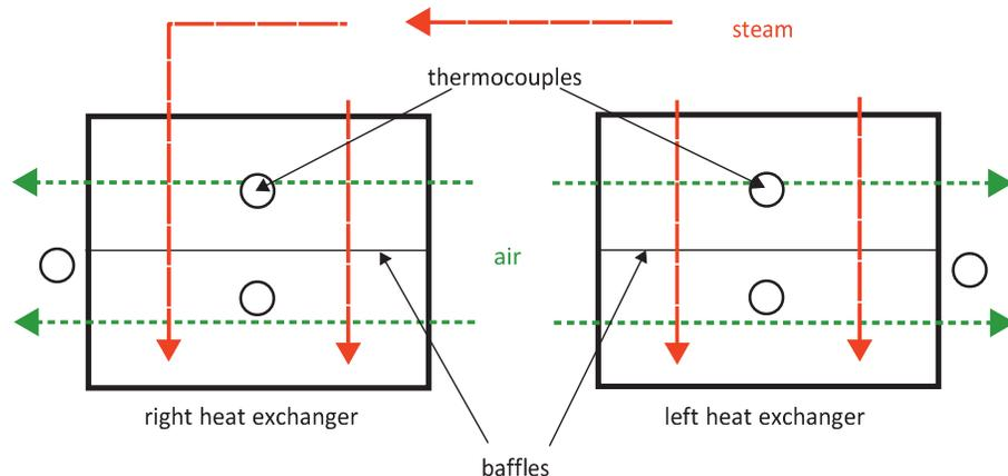
Figure 6: Scheme of the condensation hood heat exchangers – top. Two baffles included.
