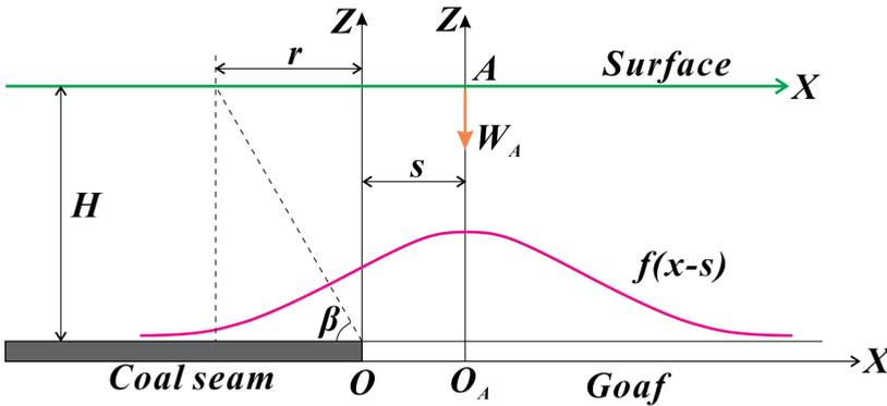
Fig. 3. Calculation coordinate system for semi-infinite extraction
