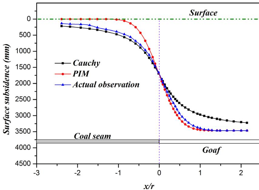
Fig. 7. Subsidence calculated using two models and observations
