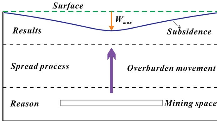
Fig. 1. The reason and process of surface subsidence
