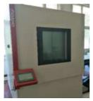
(a) Quick concrete freeze-thaw tester
