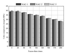
Fig. 7 Cubic compressive strength of NAC concrete specimens
