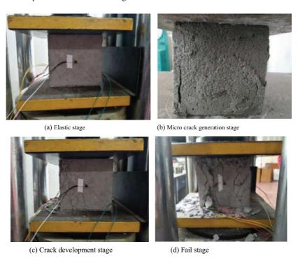
Fig. 6 Cubic compressive strength procedure of specimens
