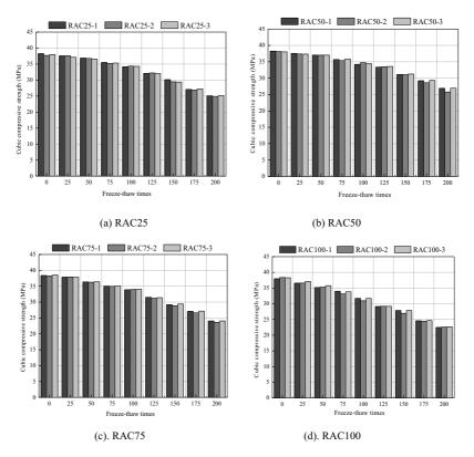
Fig 8. Cubic compressive strength of RAC concrete specimens.
