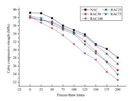
Fig. 9 Average cubic compressive strength curves
