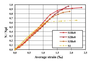
Fig. 6. Experimental N/N<sub>pl</sub> load ratio versus strain in steel cross section
