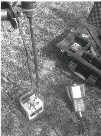
Fig. 4. Panda 2 test rig prepared for testing
