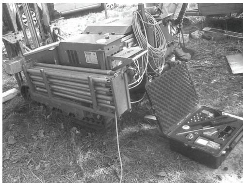
Fig. 2. CPTU test rig and Panda 2 prepared for testing
