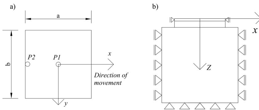
Fig. 3. a) load location b) boundary condition
