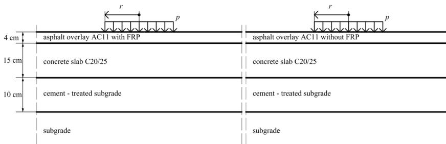
Fig. 1. Pavement structures – case S1 (left: S1-FRP, right: S1-NF)
