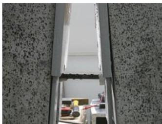
Fig. 3. Central section of an HFRP bar without bond to concrete
