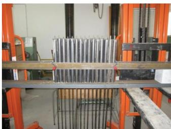
Fig. 1. A stand with unilaterally anchored HFRP bars
