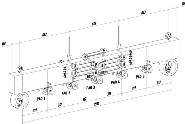
Fig. 3. Schematic location of sensors
