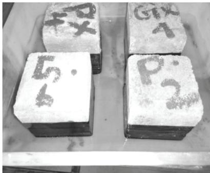
Fig 7. Sorptivity test specimen
