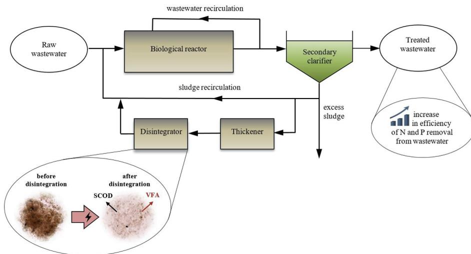
Fig. 6. Obtaining organic compounds from sewage sludge with disintegration methods and using them for supporting the removal of nutrient from wastewater
