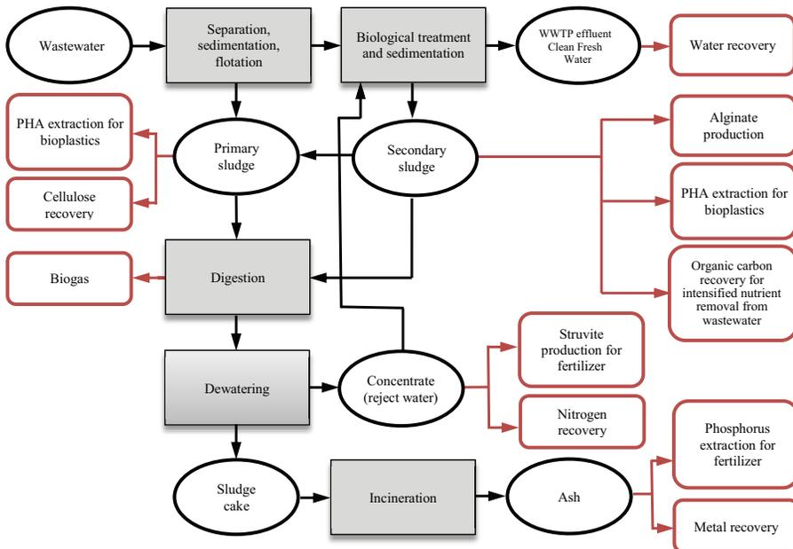
Fig. 5. Concept of energy and resource recovery in a WWTP (after [19] with own supplementation)
