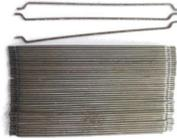
Fig. 1. Hooked-end steel fiber–3D Dramix (tensile strength = 1225 MPa, Young’s modulus =  $\pm 210,000$  MPa, length ( $l$ ) = 60 mm, diameter ( $d$ ) = 0.75 mm, aspect ratio ( $l/d$ ) = 80) [22]
