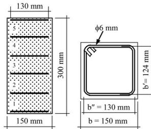
Fig. 2. Details of test specimen
