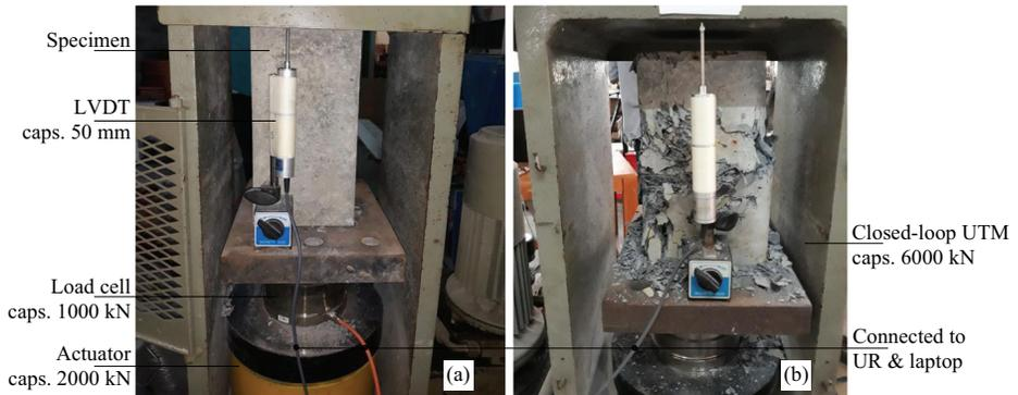
Fig. 4. Test setup: (a) front view; (b) back view.
