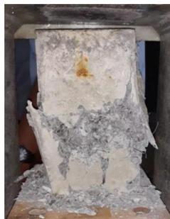
Fig. 8. Typical failure mode of specimen with  $s_h = 36$  mm failed at  $\varepsilon = 0.08$
