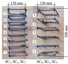
Fig. 3. Details of test specimen stirrups: SC<sub>1</sub>–SC<sub>3</sub>,  $s_h = 36$  mm; SC<sub>4</sub>–SC<sub>6</sub>,  $s_h = 52$  mm
