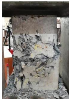
Fig. 7. Typical failure mode of specimen with  $s_h = 52$  mm failed at  $\varepsilon = 0.05$
