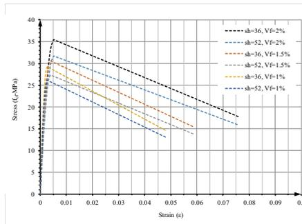
(g) Analytical curves for all specimens (SC<sub>1</sub>, SC<sub>2</sub>, SC<sub>3</sub>, SC<sub>4</sub>, SC<sub>5</sub>, SC<sub>6</sub>)
