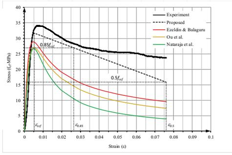
(b) Specimen SC<sub>6</sub> with  $s_h = 52$  mm,  $V_f = 2$  percent
