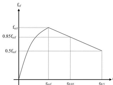
Fig. 5. Proposed stress-strain relationship of steel-fiber reinforced and confined concrete
