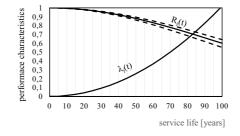
Fig. 2. Changes in the service properties and intensity of damage of masonry walls according to PRRD model.
