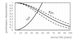
Fig. 3. Changes in the performance characteristics and damage intensity of wood ceilings
