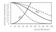
Fig. 4. Changes in the performance characteristics and damage intensity of plain roof tile
