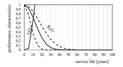
Fig. 5. Changes in the performance characteristics and damage intensity to gutters and downpipes
