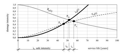
Fig. 6. Changes in the intensity of damage in an unrenovated building
