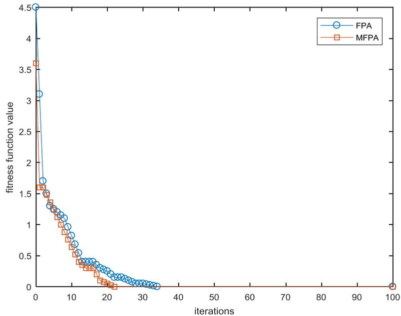
Fig. 7. Convergence curve of the FPA and MFPA under the IEEE 123 node system
