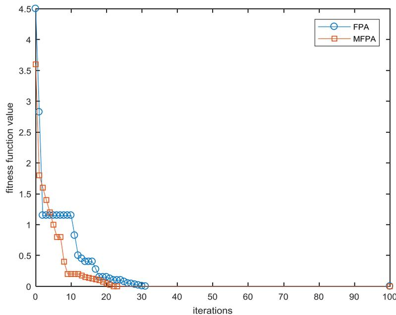
Fig. 6. Convergence curve of the FPA and MFPA under the IEEE 37 node system
