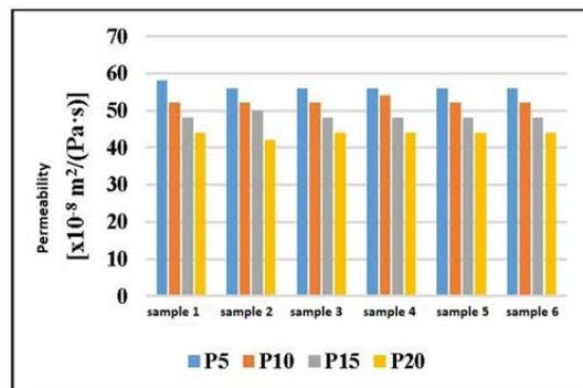
Fig. 8. Permeability of samples 1 ÷ 6 of compounds P5 ÷ P20
