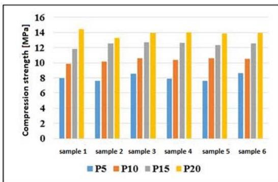
Fig. 4. Compression strength of samples 1÷6 of compounds P5÷P20
