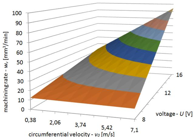
Fig. 3. Effect of circumferential velocity of working electrode – WE and voltage on machining rate -  $w_v$ . Process parameters: feed rate  $v_f = 24$  mm/min, deflection of wires  $\Delta = 0.8$  mm, wire diameter  $d = 0.5$  mm (for the central point of the experiment), the machined material – L120G13T cast steel
