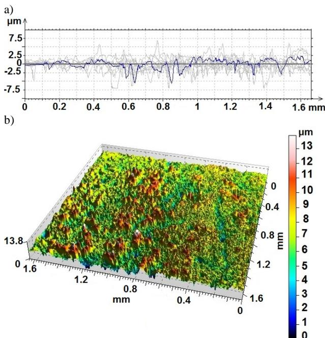
Fig. 6. Surface topography a) sample profilogram b) 3D profile map of a surface after BEDMM machining (repet. 150x); Process parameters: voltage  $U = 12$  V, circumferential velocity of WE  $v_0 = 7.1$  m/s, feed rate  $v_f = 24$  mm/min, deflection of wires  $\Delta = 0.8$  mm, wire diameter  $d = 0.5$  mm, the machined material – L120G13T cast steel
