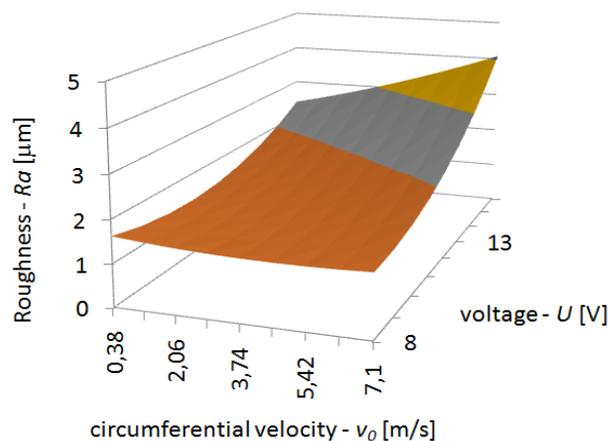
Fig. 4. Effect of the machining voltage and circumferential velocity of WE on the value of the  $R_a$  roughness. Process parameters for the central point of the experiment
