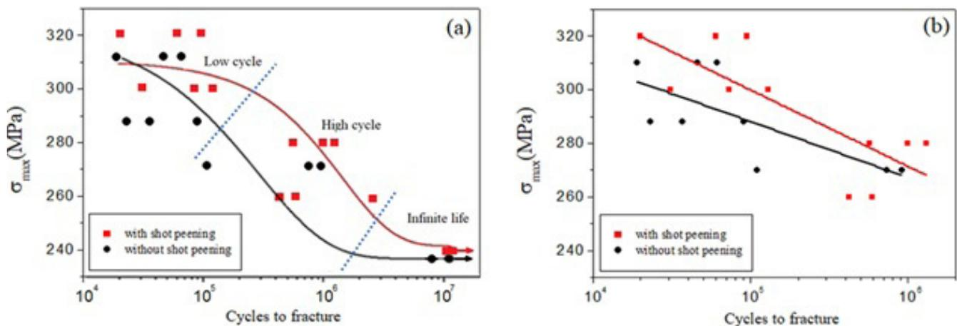
Fig. 4. Fatigue behavior of SAE 1020 steel: (a) Wöhler curves; (b) Linearized stress-life curves
