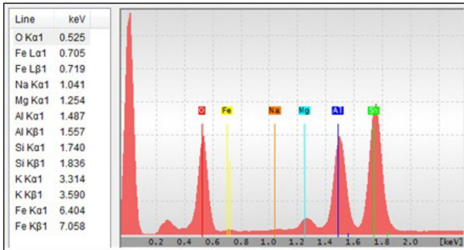
Fig. 3. Chemical composition of the inclusion (EDX-SEM)
