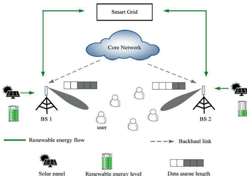
Fig. 1. Structure of cooperative energy multi-layered heterogeneous system powered via current grid and alternative resources
