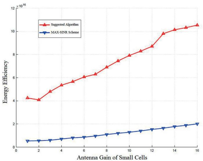
Fig. 6. Energy efficiency versus the mmWave small cell antenna gain
