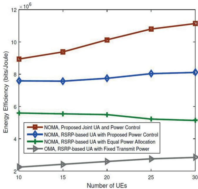
Fig. 7. Comparison of user association/resource allocation approaches from energy efficiency vs user equipment perspective
