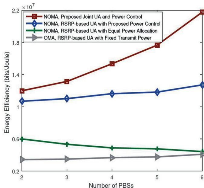
Fig. 8. Comparison of user association/resource allocation approaches from energy efficiency vs pico base stations perspective
