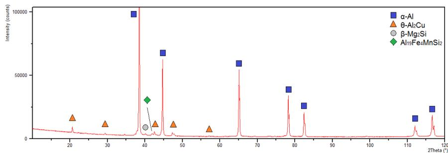
Fig. 6. X-ray diffraction analysis of AlCu4MgSi alloy ingots
