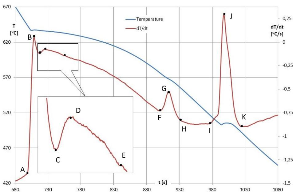
Fig. 3. Thermal and derivative analysis curves for the studied alloy. The cooling curve  $T = f(t)$  and the crystallization curve  $dT/dt = f(t)$  with indicated characteristic points. Full description in the text
