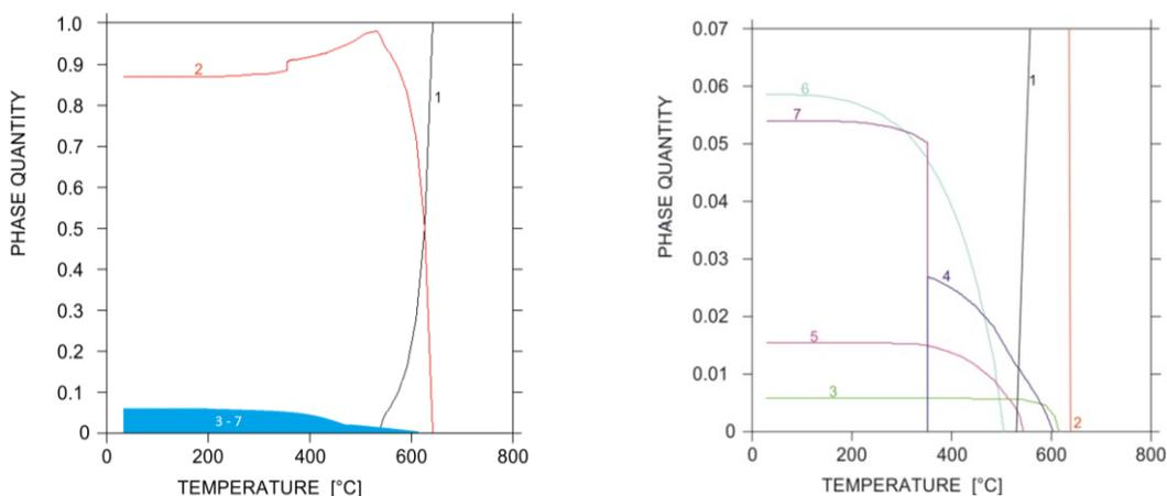
Fig. 2. Results of numerical simulation for the studied alloys. Volume fraction of occurring phases in function of temperature. Full diagram (left), magnification (right). 1 – liquid, 2 –  $\alpha$  phase, 3 –  $\text{Al}_{13}\text{Fe}_4$ , 4 –  $\text{Al}_6\text{Mn}$ , 5 –  $\text{Mg}_2\text{Si}$ , 6 –  $\text{Al}_2\text{Cu}$  ( $\theta$  phase), 7 –  $\text{Al}_{12}\text{Mn}$
