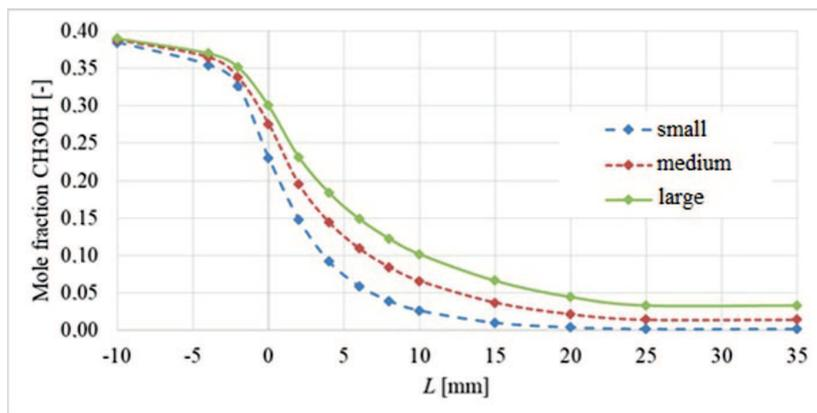
Figure 7: Mole fraction of CH<sub>3</sub>OH for different scale factor for assumed geometry. Thermocatalytic reaction area is located between  $L = 0$  mm and  $L = 25$  mm.
