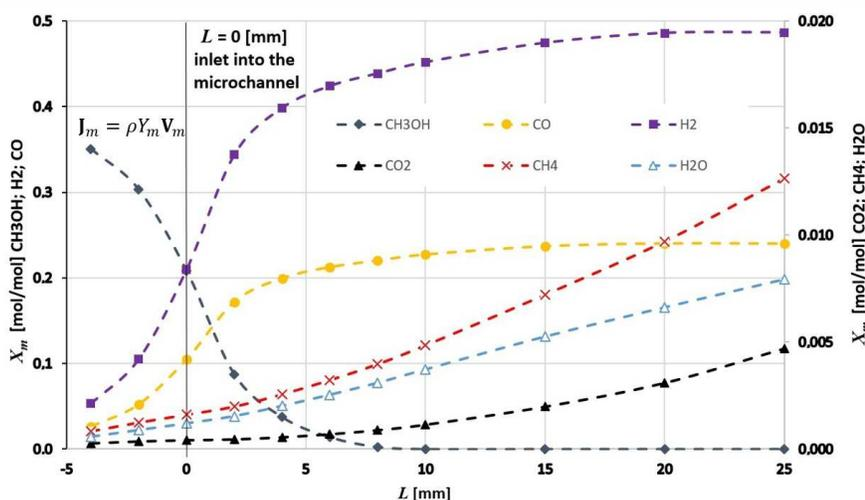
Figure 5: An averaged cross-sectional mole fraction of  $\text{H}_2$ ,  $\text{CH}_3\text{OH}$ ,  $\text{CO}$ ,  $\text{H}_2\text{O}$ ,  $\text{CH}_4$ , and  $\text{CO}_2$  as a function of the reactor length  $L$ . Thermocatalytic reaction area is located between  $L = 0$  mm and  $L = 25$  mm.
