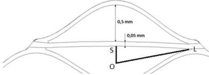
Figure 2: Cross-section of the microchannels in the honeycomb with highlighted characteristic dimensions of thermocatalytic reactor, where short straight  $|OS| = 0.184$  mm and long straight  $|OL| = 0.834$  mm.
