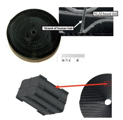
Figure 1: The alloy foil package based on the  $Ni_3Al$  intermetallic phase rolled into a honeycomb with zoomed foil and geometry of the eight single microchannels beginning at inlet into the package and terminating at the outlet from the package.
