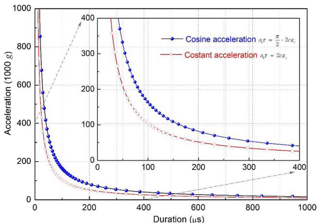
Fig. 4. Limit curves for the cosine and constant acceleration calibrations.
