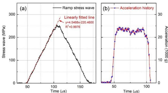
Fig. 2. A linear ramp wave and the corresponding acceleration wave.
