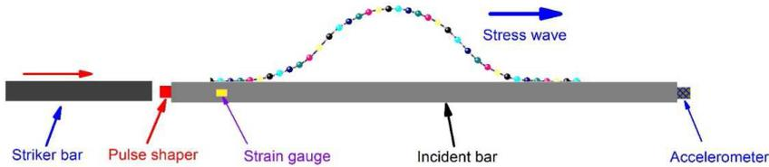
Fig. 1. A schematic of the Hopkinson bar calibration system.
