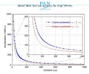
Fig. 4. Limit curves for the cosine and constant acceleration calibrations.
