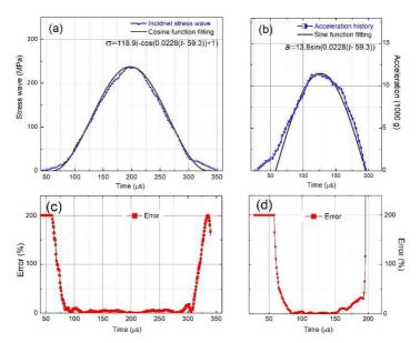
Fig. 3. Comparison and error analysis of the loading stress wave with a cosine function and the corresponding acceleration wave with a sine function, obtained from the experimental and fitting results.
