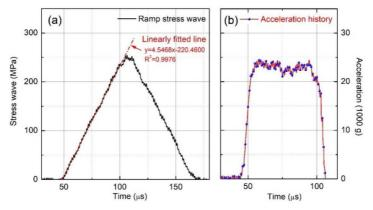
Fig. 2. A linear ramp wave and the corresponding acceleration wave.
