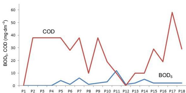
Fig. 9. Variation of BOD<sub>5</sub> and COD in the M'zab valley; P1–P18 = measurement points as in Fig. 3; source: own study
