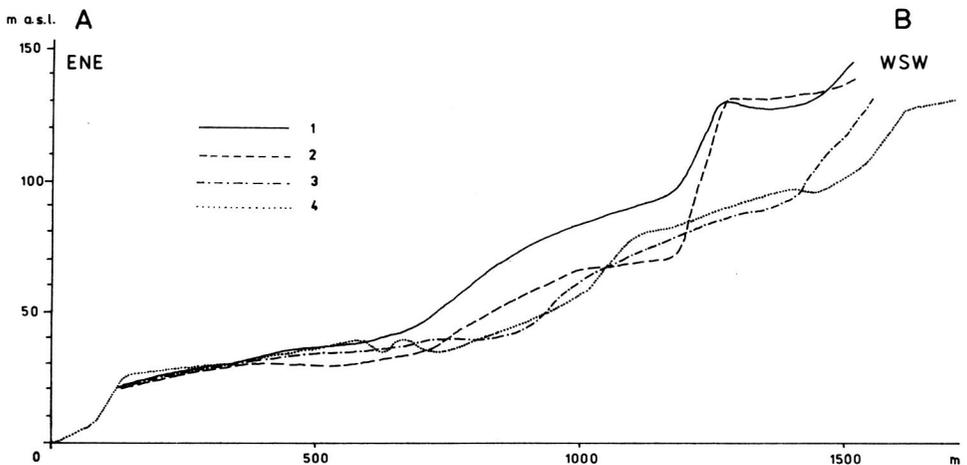
Fig. 2. Morphological profiles across raised marine beaches on Calypsostranda along the line A—B (cf. Fig. 1). 1 — altimeter route, 2 — clisimeter route, 3 — profile from a photogeological map at a scale of 1:10,000, 4 — profile from direct readings on air photos
