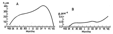
Fig. 2. Variation of A — mean depth of snow, and B — density of snow in the Arctic Basin; after Vowinckel and Orving (1973)
