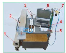
Fig. 7. The detail of the measuring apparatus of gas evolution of moulding and core sand mixtures. 1-furnace controller, 2-Mars furnace, 3-prussure sensor, 4-data bus, 5-voltage source for the bus, 6-PC, 7-pressure vessel with nitrogen gas (N<sub>2</sub>).
