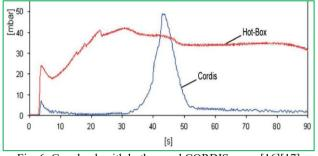
Fig. 6. Gas shock with hotbox and CORDIS cores [16][17]
