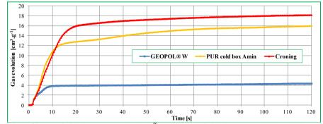
Fig. 10. Gas evolution of inorganic binder system GEOPOL<sup>®</sup> W and organic binder systems PUR cold box amin and Croning.
