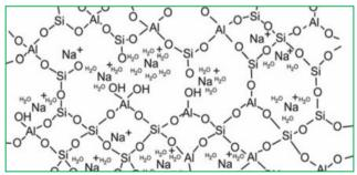
Fig. 2. Scheme and model of inorganic polymer by Davidovits [1] and updated by Barbosa [6] and later by Rowles (bottom) [7]
