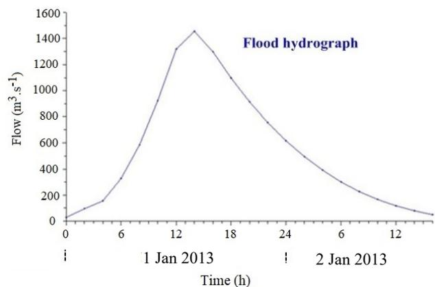
Fig. 5. Dam inlet flood hydrograph; source: own elaboration
