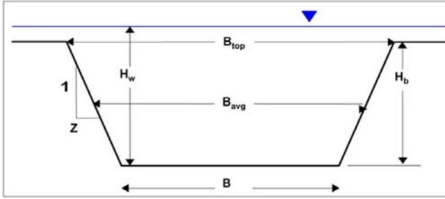
Fig. 6. Breach profile type; source: own elaboration
