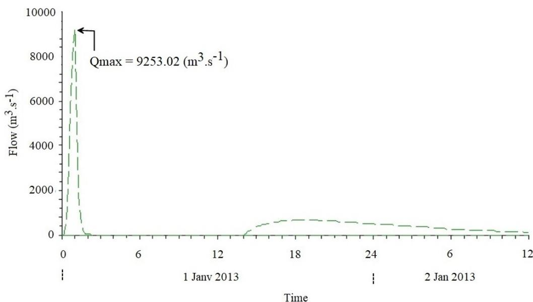
Fig. 14. Breach hydrographs at dam; source: own study
