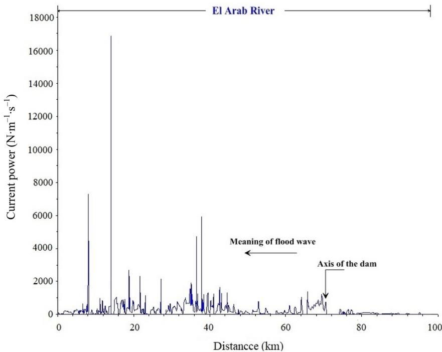
Fig. 12. Water current power of the flood wave; source: own study
