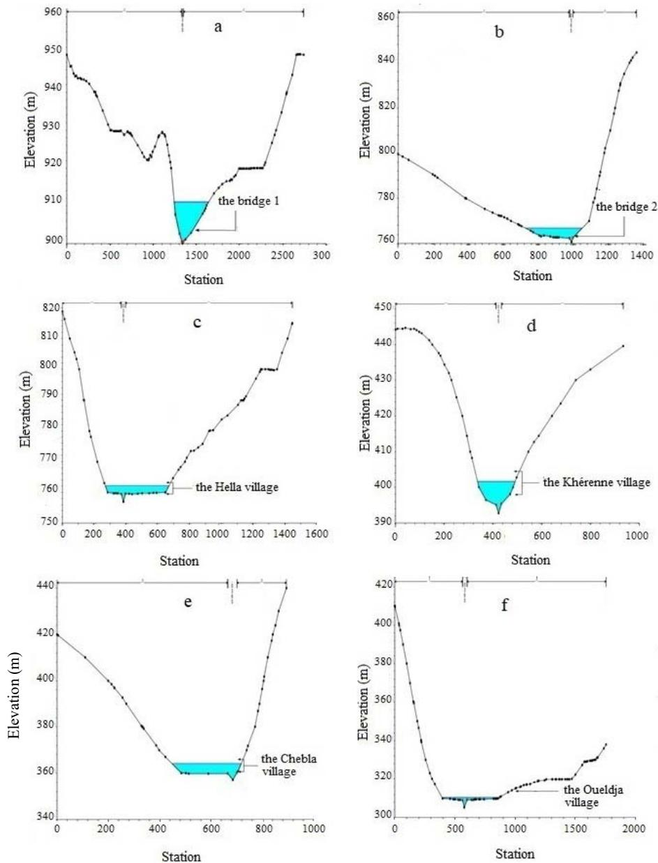
Fig. 15. The water level after the failure at: a) the bridge 1, b) the bridge 2, c) the Hella village, d) the Khérenne village, e) the Chebla village, f) the Oueldja village; source: own study
