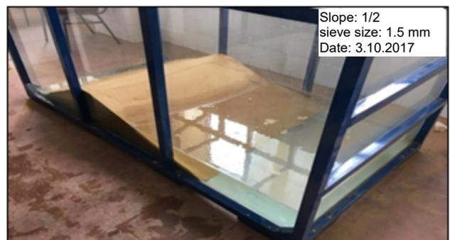
Fig. 6. Seepage water of the experimental model dam; source: own study
