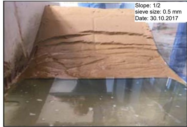
Fig. 14. Failure of the experimental model dam, crest width –  $B = 5$  cm; source: own study
